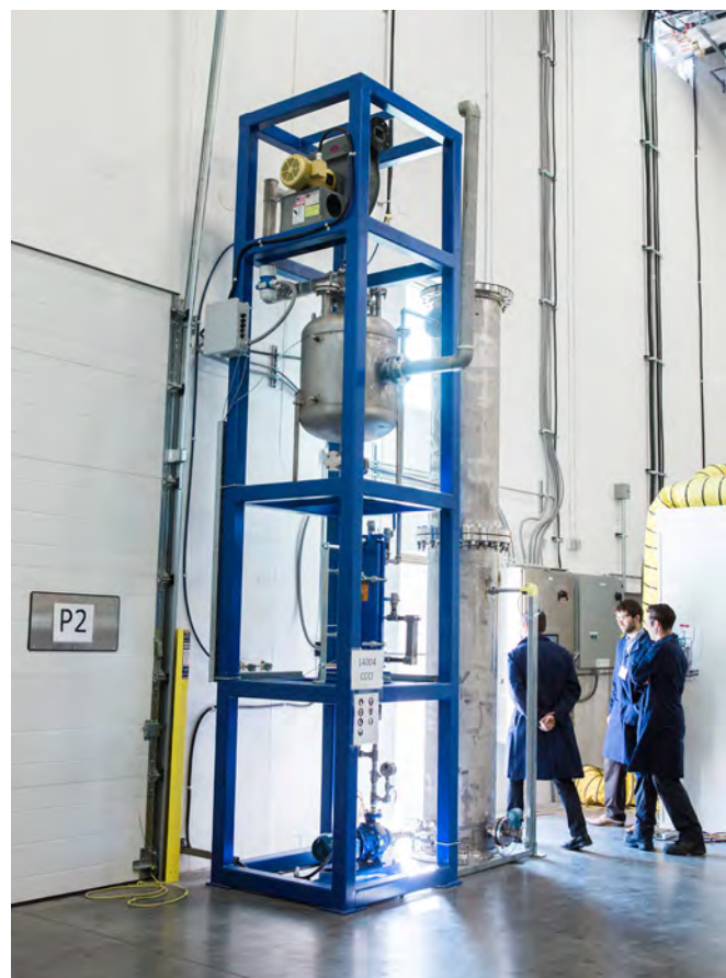
Flue gas conditioning unit at CMCR's carbon capture and conversion facilities in Vancouver.
